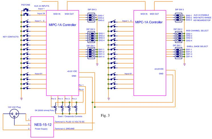
MIPC-1A-HV switch commons are connected to PLUS 7 to 17 Volts D.C. MIPC-1A Switch Commons to GROUND.
