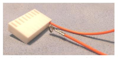
After crimping, check to make sure the two sets of crimp tabs are securely crimper with the rear set around the insulation and the front tabs around the wire.
