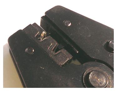
Place the terminal in the crimper with the crimp tabs facing the AWG 24-30 Gage Wire numbers. After placing the terminal in the crimper jaws, squeeze the handle until you hear one or two clicks. This will hold the terminal in place.
