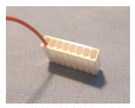
When inserting the wire and terminal in the connector housing, verify that the terminal locking tab is facing the small slot for each position. Slide the wire in until the locking tab clicks in place.
