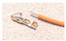
Strip the insulation about 1/8". Insert the wire in the terminal to be crimped and squeeze the crimper handles together.
