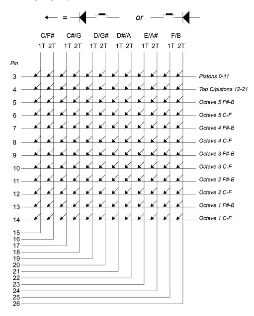
Mode 2 can also be used for connection to an Allen MOS keyboard. These use a  $6 \times 11$  matrix of switches, which is essentially the same as our mode 2 without second touch.
