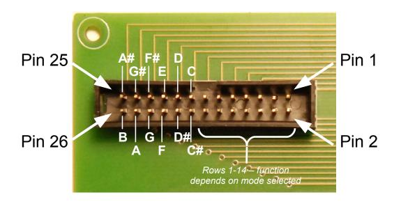
The unit automatically reads each "row" in turn, by switching one row select line at a time to logic 0 (0v). When this happens, keys which are pressed in the relevant octave will be read as 0 and keys which are not pressed will be read as 1 (5v). The entire matrix is read approximately 100 times per second.
