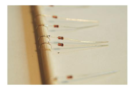
The ends should be soldered so that the loop cannot become undone. Try not to wrap the anode lead too tightly around the dowel; you will find the next step much easier if you can slide the diodes along the dowel without too much resistance.
