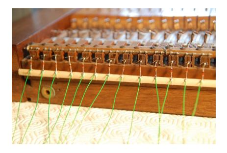
Next, solder each wire to the diode twelve positions to the right of it. In this way, you join up all the C's, all the C#'s, and so on.
